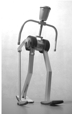
Figure 4.1 A passive walker: a robot that uses gravity and clever mechanics to balance and walk without any motors. (Photo by Jan van Frankenhuyzen, courtesy of Delft University of Technology)
