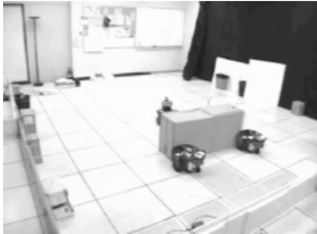
Figure 20.1 A robot team collectively pushing a box; one robot (behind the box) is the watcher, which steers the team toward the goal, while the two others are the pushers. In this case, it takes three to tango, or at least to push this particular box. (Photo courtesy of Dr. Brian Gerkey)
