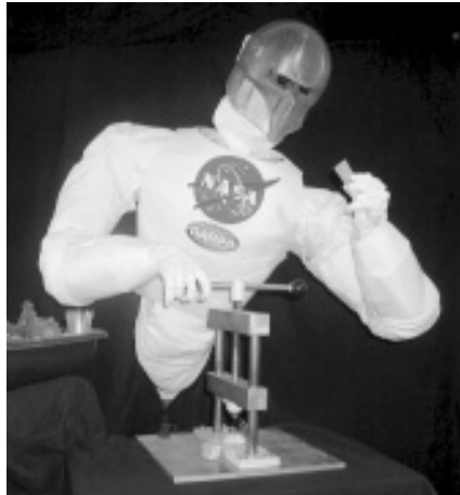
Figure 22.6 NASA's Robonaut, the first space robot with a humanoid torso. (Photo courtesy of NASA)
